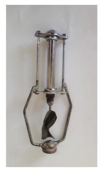
This sprinkler is an example of local ingenuity and craftsmanship. A bicycle pedal frame is used to produce a rotor that is equipped with ball bearings. This is probably done to try and answer to the problem of fast wear and tear of other sprinklers. As such, this is a brilliant idea. Unfortunately its' implementation was not very successful.
