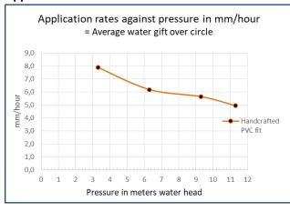
The application rate of this sprinkler is relatively high compared to most other sprinklers. This is due to the fact that the radius of the sprinkler is limited. It appears that the rotor blade is not very effective in spreading the water.
