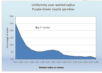
This graph shows that the uniformity of this sprinkler is not good at 0.6 Bar.
