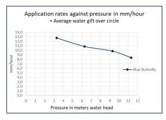
The application rate of the blue butterfly is 11 mm/hour at 0.6 Bar. The iron butterfly has an application rate of 4 mm/hour at 0.6 Bar.
