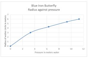
This indicates that the Blue Iron butterfly is spraying much more water over a more limited area, compared to the Iron Butterfly. This can be seen back at the application rate.
