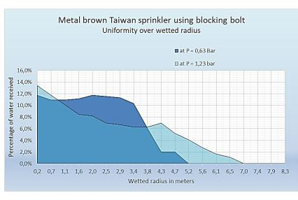
When using the blocking bolt, the uniformity of application is good, especially at P = 0.63 Bar. Over the longest part of the circle, the water application rate is between the 11% and 12% of all water sprayed. At P = 1,23 Bar, uniformity is lower, with a higher proportion of the water falling in the first meter.
