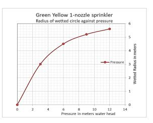
The flow is a little bit less than the flow of the yellow butterfly sprinkler. Also, the wetted radius is smaller. It gives a radius of 5,5 m at a pressure of 1 Bar, whilst the yellow butterfly gives a radius of 8 m at a pressure of 1 Bar. The advantage of this sprinkler is that the flow is adjustable. We did not test this sprinkler at different knob positions. Probably, also the radius will vary with different knob positions.
