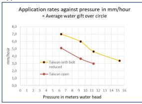
As the water flows in the two bolt positions are equal, the average application rates depend only on the sizes of the wetted circles.
