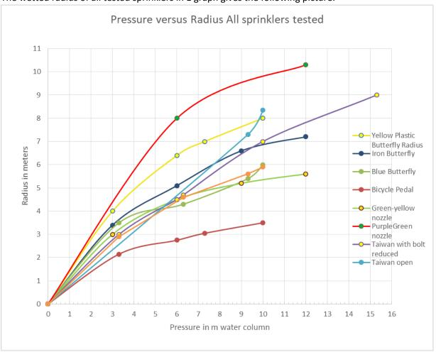
Generally, a large wetted radius is to be preferred, because this reduces the need for replacing the sprinkler often. A larger wetted radius usually also implies a low average application rate.
