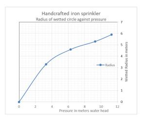
The sprinkler flow is relatively low, indicating a small nozzle size. At 6 m water head this sprinkler has a flow of 6.6 l/min, which is less than the yellow butterfly sprinkler.
