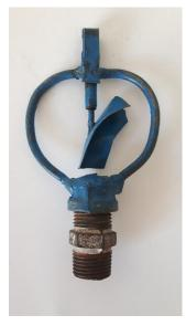
This is a locally produced version of the iron butterfly sprinkler. Note that the rotator is mounted on top, but not attached to the sprinkler base. The rotator is less smooth, and bending seems to be done by hand (using tools). It was painted blue by the manufacturer.
