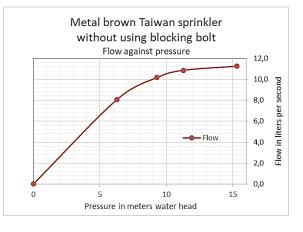
As expected, the flow against pressure is equal, because the flow at certain pressure largely depends on the size of the nozzle opening and this did not change. The bolt is influencing the wetted radius, and the way the water spreads over the wetted circle. With the bolt blocking, the wetted radius at 1 Bar is 6 meters, against 7.6 meters without blocking.
