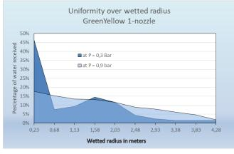
As can be seen in the graphic, the sprinkler does not operate well under the low pressure of 0.3 Bar. At this pressure, the uniformity of this sprinkler is not good at all. Pity we did not test the uniformity at 0,6 Bar. It can be concluded that this sprinkler should not be recommended as low pressure sprinkler.
