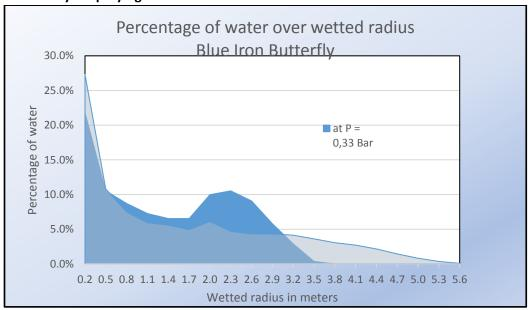
The graph above shows the uniformity of spraying over the wetted area at P = 0.33 (dark blue) and P = 0.93 Bar (light blue). The same pattern can be seen for all 3 butterfly sprinklers. At the lowest pressure, the uniformity is less than at higher pressure; the water application right next to the pole is very high, and going further from the pole, this drops and then rises again to a peak.
