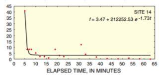
This implies that in the first 5 minutes, the soil is able to absorb a lot of water. This graph shows what happens if indeed all water absorption capacity is supplied: the top layer of the soils is saturated after a short time, and after this, the infiltration rate reduces to a stable (approximately) 3 mm per hour.
